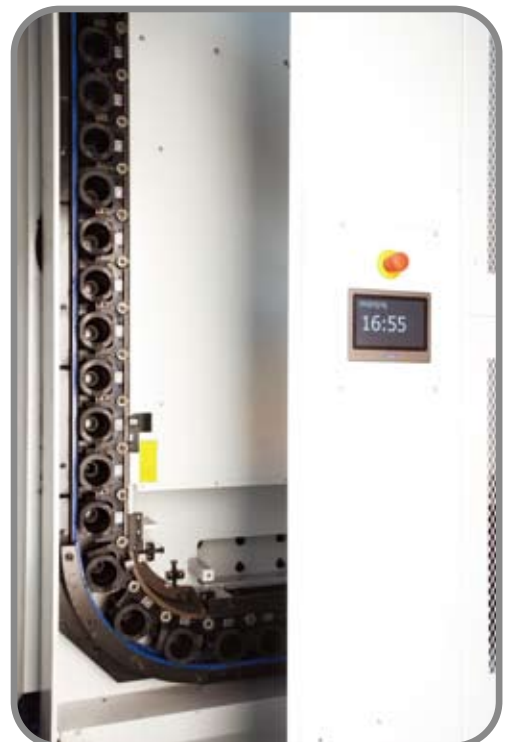
Tools can be inserted at side door where a small control panel for easy tool selection.
