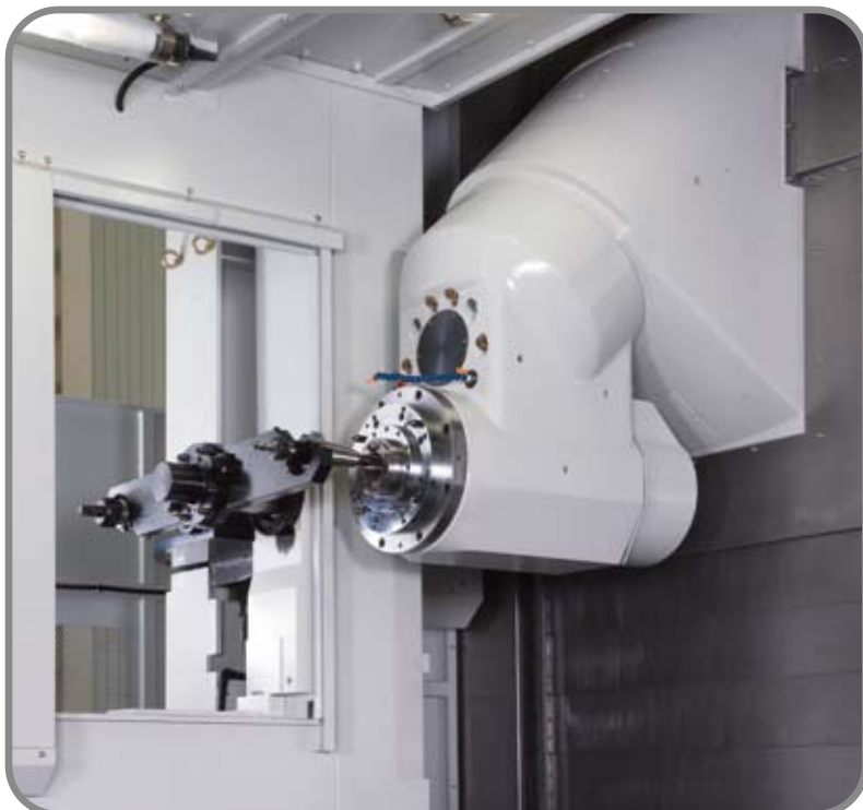
Tools exchange automatically when spindle at horizontal position.
